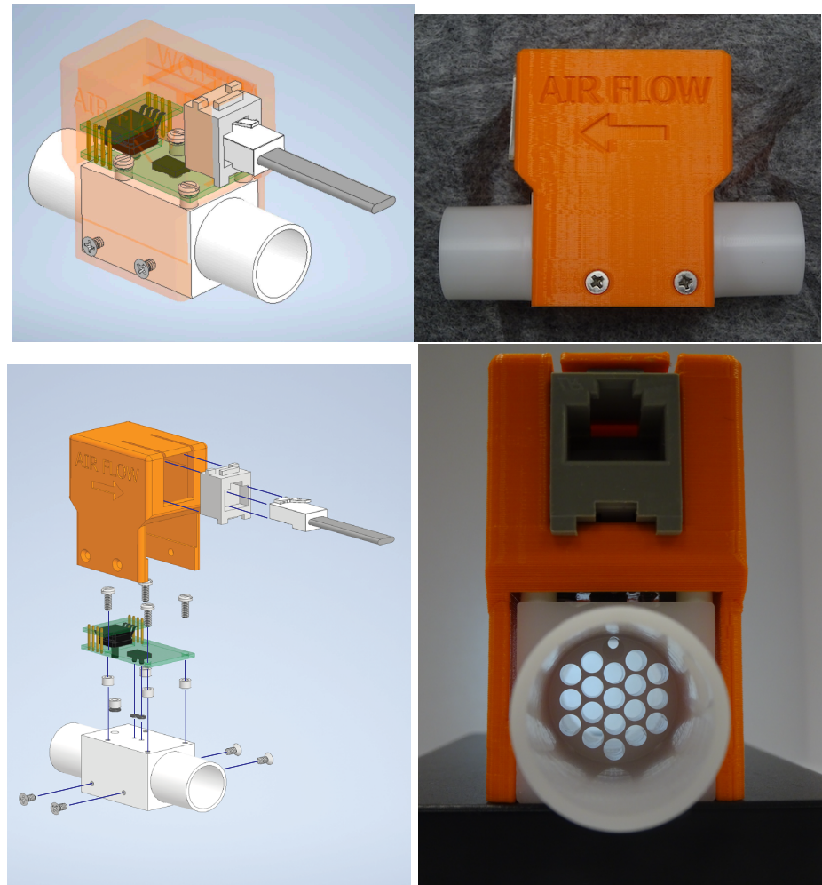
Fig 3. Flow-sensor assembly. A flow and pressure sensor are exposed to the flow element. The electronic sensor elements are mounted on circuit boards that connect to an external RaspberryPi controller via a standard RJ-45 jack.
